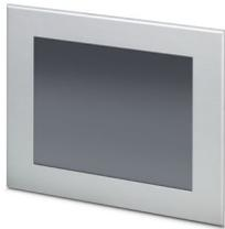
Pannello tattile, 30.7 cm / 12.1"-TFT display (analogico-resistivo (poliestere)), 800 x 600 pixel (SVGA), 262144 colori, Xscale® PXA320, 806 MHz, 2x USB Host 1.1, 1x CompactFlash®, 1x Ethernet (10/100 MBit/s), RJ45, Windows® CE 6.0, Visu+ / AX OPC Server, senza sistema bus.
