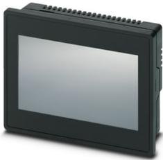
Webpanel, 10.92 cm / 4.3"-TFT Display (analog-resistiv), 480 x 272 Pixel (WQVGA), 16,7 Mio. Farben, i.MX 6DualLite, 1 GHz, 1x USB 2.0, 1x Ethernet (10/100 MBit/s), RJ45, Yocto/Linux®, QT-Browser, ohne Bussystem.
