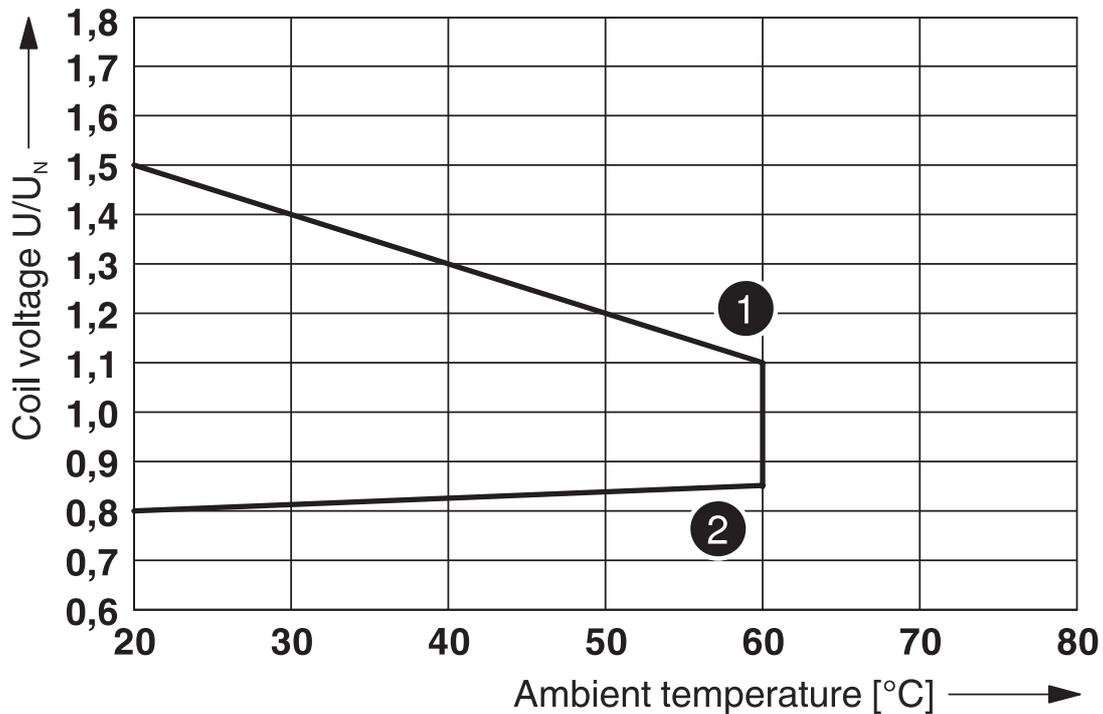
① Maximum continuous voltage at limiting continuous current = 6 A
