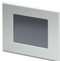
Web panel, 17.8 cm / 7"-TFT display (Touchscreen industrial resistente), 800 x 480 pixel (WVGA), 65536 cores, Arm9™, 184 MHz, 2x USB Host 2.0, 1x Ethernet (10/100 MBit/s), RJ45, Windows® CE 5.0, MicroBrowser, sem sistema de bus.
